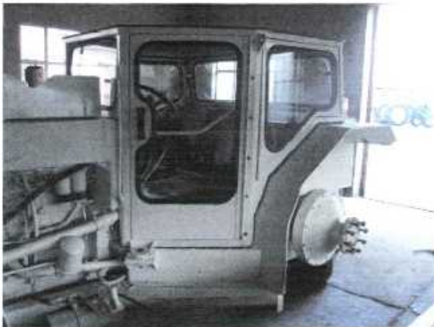
Figure 1. Tractor with enclosed cabin – manufactured for use in the mining industry.
