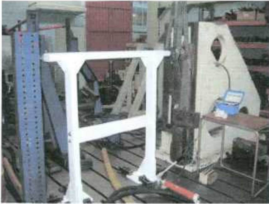
Figure 2. ROPS under load during the lateral load test.
